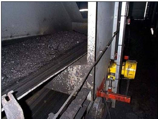
Rulmeca Motorized Pulley drives belt at discharge end.
